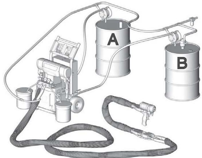
Two-component foam proper set up – Isocyanate (A); Resin (B)
