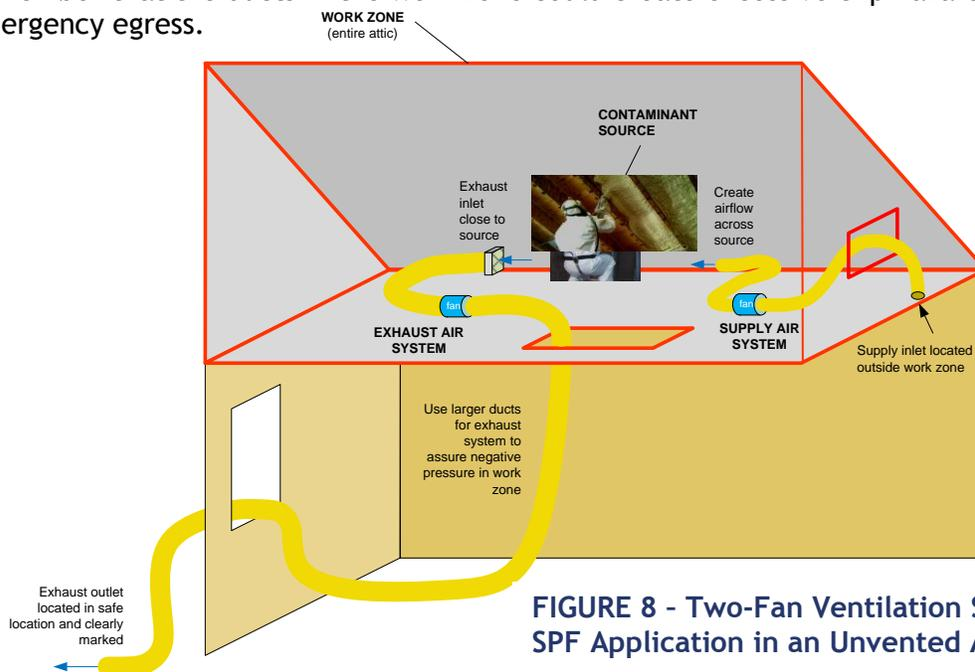
FIGURE 8 - Two-Fan Ventilation System for SPF Application in an Unvented Attic
